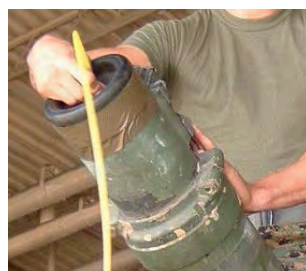
Tube Strip being inserted into a barrel.
